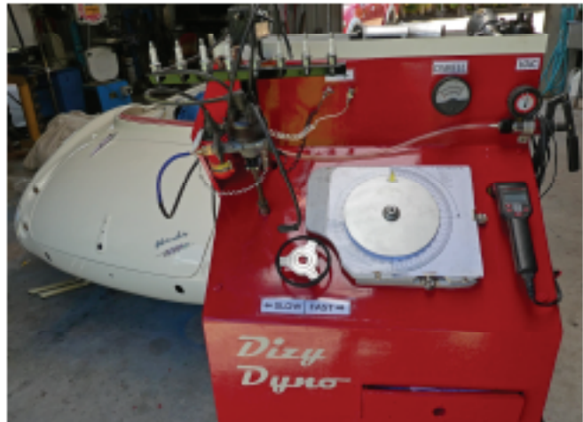
Distributor test bench for analysing distributor performance.
